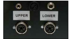
Rear-panel showing photo-detectors connectors.
